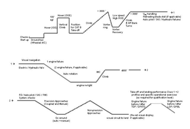
It is proposed that the existing typical test profiles for FSTD aeroplane and helicopter are provided in GM with the reasoning that such profiles are indicative, and the operator/authority may define different ones, considering the specificities of each FSTD and the performance of the aircraft simulated.
