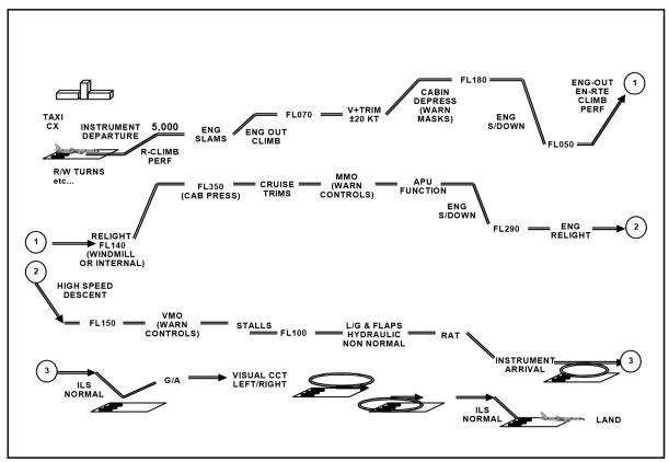
(b) Typical test profile for an FSTD helicopter:
